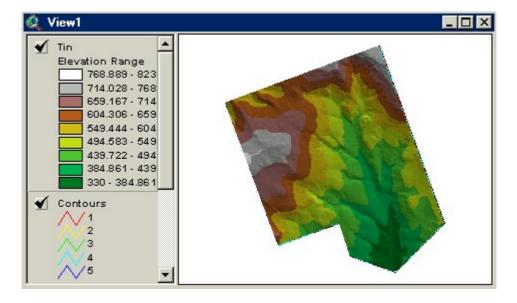
Lest's simplify DTM converting it to a Grid. Select Theme/Convert to Grid from the menu and after setting the location and name of the grid, set the parameters as follows. You must set first the resolution and then select the output grid extent and the number of rows, columns are recalculated. Finally add the new grid to our view.
