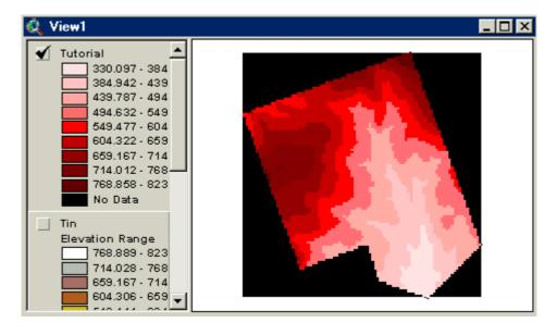
We have to remove sinks from the DTM for hyrologic modeling. Let's load the Hydrologic modeling
