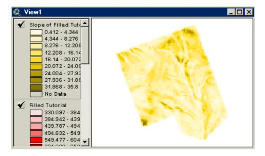
Let's generate a flow directions grid from the Filled Tutorial grid. This grid shows the on surface water flow direction from one cell to one of the eight neighboring cells. Make the Filled Tutorial the active theme and select **Hydro/Flow Direction** from the menu. Directions are coded
