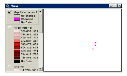
Lest's derive slopes from the DTM. Make the Filled Tutorial the active theme and Select **Surface/Derive** slope from the menu. We get another grid, the values are a slope in degree.
