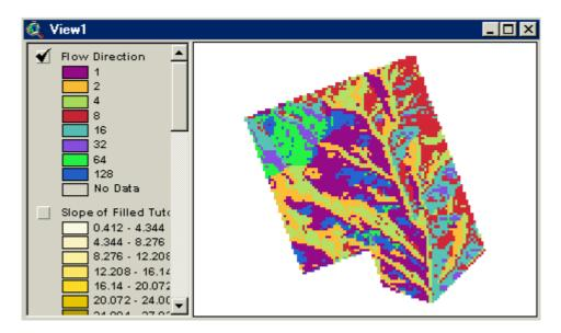
Now we will use flow directions to find the creeks, streams. We can accumulate flow directions, the number of cells from which water flows to a cell are counted during the accumulation. Make the Flow Direction theme the active theme and select **Hydro/Flow Accumulation** from the menu. We get the Toka creek.
